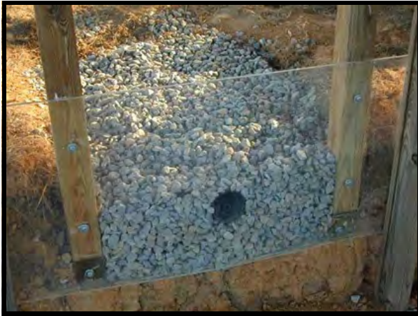
Conventional gravel trench with 4" inch perforated pipe.
