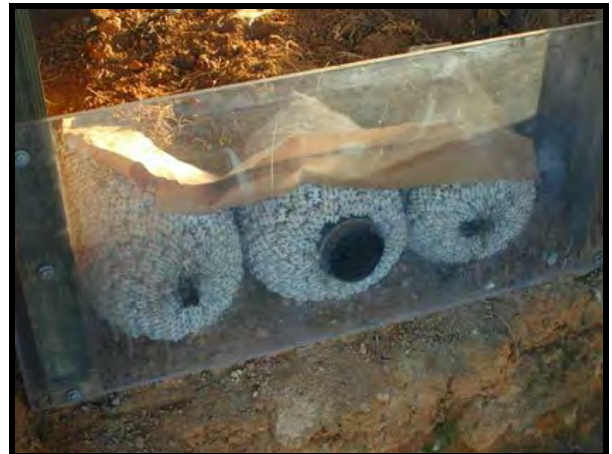
Perforated flexible 4" inch pipe (Expanded Polystyrene Bundles).
